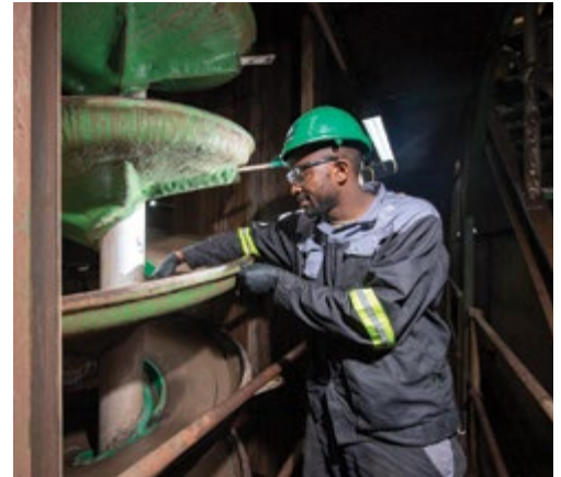
Manganese stockpile material was tested using the Multotec UX7 ultra-fine spiral concentrator for roughing and scavenging phases, and the Multotec SC21 five-turn spiral for the cleaning phase.
