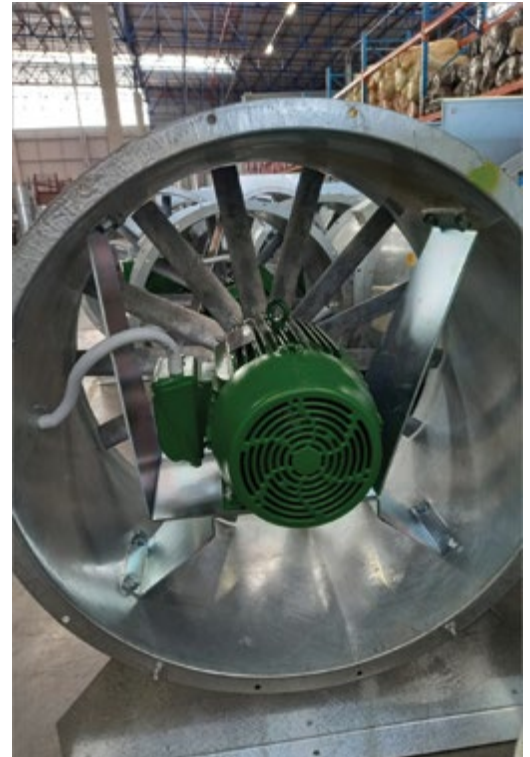
A WEG motor being installed on a fan.
